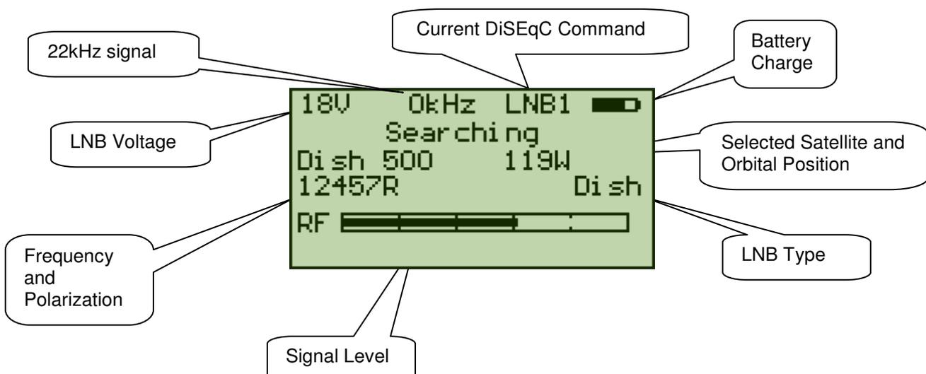
The signal level will increase on the signal bar if any satellite signal is detected. If the beeper is enabled, then the pitch of the beeper will increase with signal strength. Once the instrument locks on a satellite transponder, the display is changed. Once locked on a transponder, the SNR (signal to noise ratio) bar and the Quality bar (derived from BER - bit error rate) are displayed.
