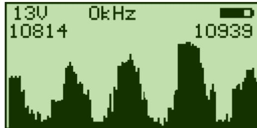
On entry, the spectrum display shows a 125MHz band centered on the current Satellite Search satellite.
