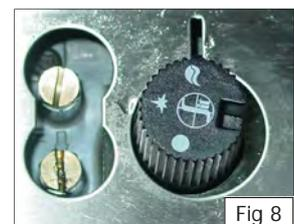
**NOTE:** As a safety precaution all Blue Seal 'Fast-Fri' Fryers feature an Over-Heat Control, which will 'Turn Off' the fryer should there be a thermostat failure and the oil temperature reaches over 220°C.
