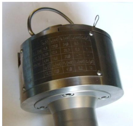
GasClam identification plates with intrinsic safety specifications.
