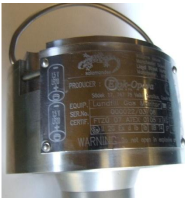
GasClam identification plates with intrinsic safety specifications.
