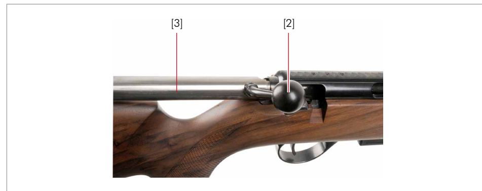
Fig.29 Pivoting the bolt handle downwards
