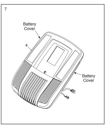
8. While a second person holds the Console (4) near the Upright (2), connect the wires on the Console to the Main Wire (53) and to the Frame Pulse Wires (42).
