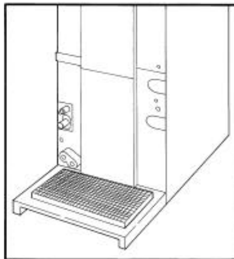
Fig. 5—Removing Filter from Fan Coil Unit
