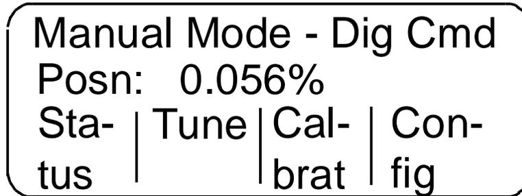
The HOME menu has selections of **STATUS**, **TUNE**, **CALIBRATE**, and **CONFIGURE**. Each of these menus has several sub-menus. The bottom two lines define the function keys that control the individual menus. The top two lines in the display are user configurable and may not look like Figure 1.
