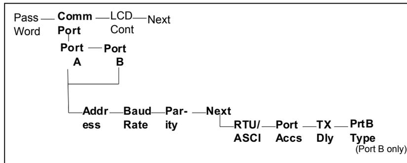
**Port A / Port B** - This option allows the user to configure Port A and Port B independently. By selecting Port B there is an added menu item to be able to select which input from Port B to use.
