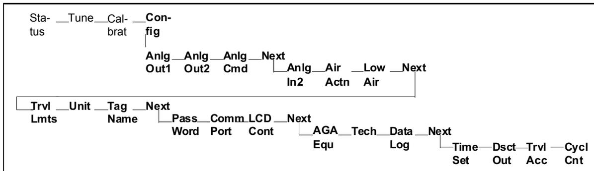
**Analog Out 1** - This option configures the first analog output channel. Select a variable from the list using the NEXT and PREVIOUS function keys on the menu. You will then be asked for a full scale output value in your selected user units. (This is the process value that corresponds to 20 mA.) The last step is to enter the offset or Zero output value in your selected user units. (This is the process value that corresponds to 4 mA.) Available output variables are:
