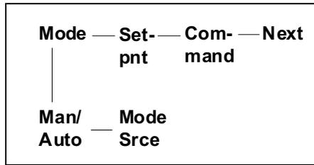
**Man/Auto** - This option selects or changes the operating mode if the mode source has been set to digital. If the mode source is set to Remote or Discrete, the mode can only be changed using the discrete input or the remote register. In Manual mode the unit operates as a normal control valve, positioning the valve according to its current command signal.
