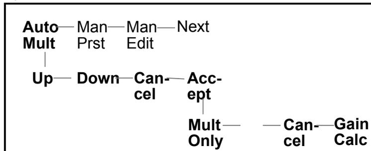
Displayed on Row 1 will be the multiplier value with selections from A to H. These are represented in table 2. These values are multiplied by the final gain to allow the user to adjust the responsiveness of the valve.
