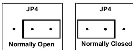
**Discrete Input Range Selection** - On the lower right hand side of the electronic board assembly on the bottom board is a six position jumper labeled “JP4.” There are 2 jumpers that must be moved together to set the voltage input range. The jumpers are oriented vertically and with both jumpers in the upper position the input is set to trigger on 120V AC or DC. With both jumpers in the lower position the input is set to trigger on 24V AC or DC.
