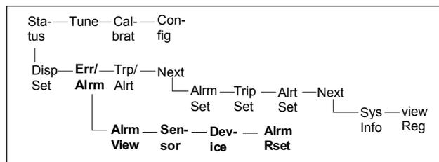
**Alarm View** - Allows the user to view any current alarms using the NEXT or PREVIOUS function keys. Possible alarms are:
