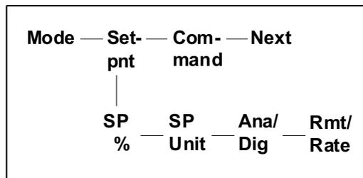
**Setpoint %** - Allows the direct input of the controller setpoint as a percentage of maximum, as setup with the process variable, provided the unit is in the Auto mode with the digital setpoint selected.
