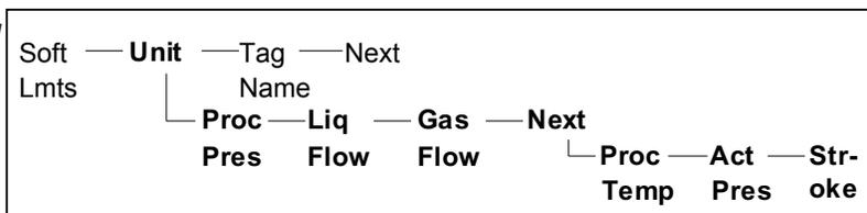
**Process Pressure** - This option sets the process pressure engineering units for the StarPac 3 system. Use the NEXT and PREVIOUS function keys to select units from the following list:
