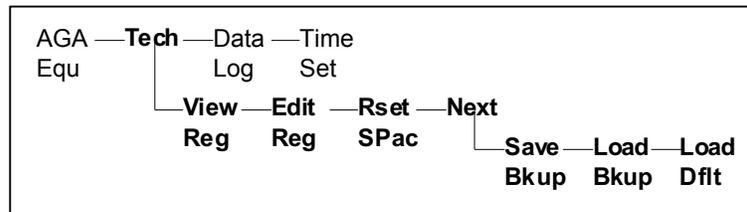
**View Register** - This option allows you to view any integer or floating point Modbus register. A register map is located in the appendix. (String registers cannot be viewed with this function; however, they can be viewed by using the StarTalk software.)
