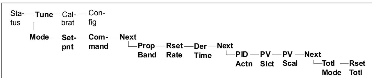
**Setpoint User Units** - Allows the direct input of the setpoint in the configured engineering units, provided the unit is in Auto mode with the digital setpoint selected.
