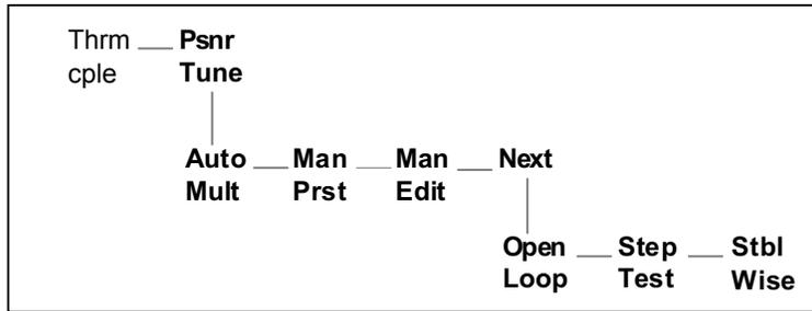
**Auto Tune / Multiplier** - This option allows the user to adjust the gain multiplier and/or commands the positioner to automatically compute the gains to be used by the positioner based upon the stroke time of the valve.
