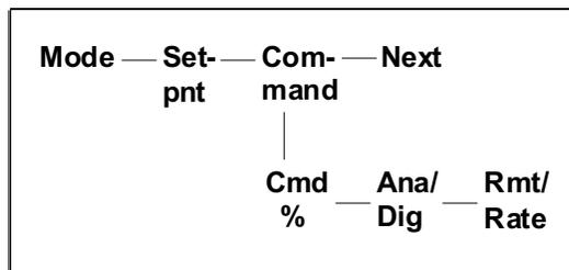
**Command %** - Allows the direct input of the valve position command as a percentage of valve travel. Zero percent is closed and 100 percent is open--provided the unit is in Manual mode with the digital command selected.
