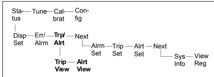
**Trip View** – Trips are conditions that take the StarPac 3 system out of service and drive it to a fail condition.
