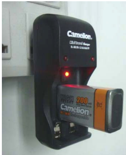
Figure 3-14 Charging NI-MH battery
