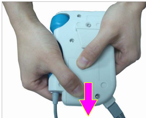
Figure 3-1 Opening battery compartment
