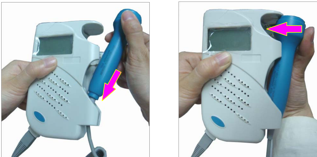
Figure 3-5 Placing the probe
