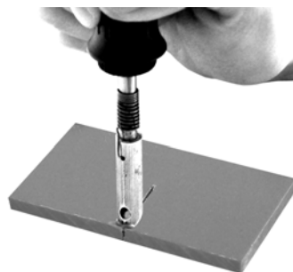
Tacking plastic parts with stitching action
