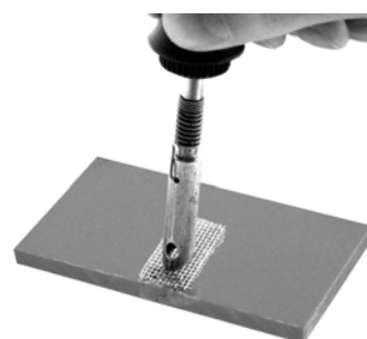
Sink in the metal mesh with heat and gentle pressure
