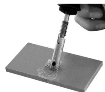
Cover the mesh with melted plastic
