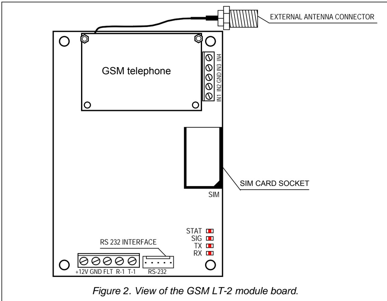
Figure 2. View of the GSM LT-2 module board.
