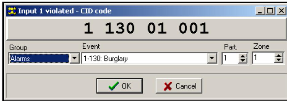
Figure 12. View of the CID code generator.
