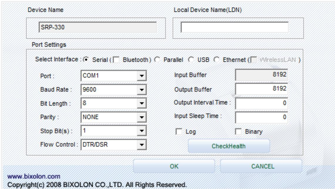
3) Set the communication environment of the connected printer and click “SAVE” or “OK” button.
