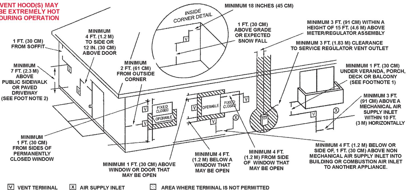
1. PERMITTED ONLY IF VERANDA, PORCH, DECK OR BALCONY IS FULLY OPENED ON A MINIMUM OF TWO SIDES BENEATH THE FLOOR.
