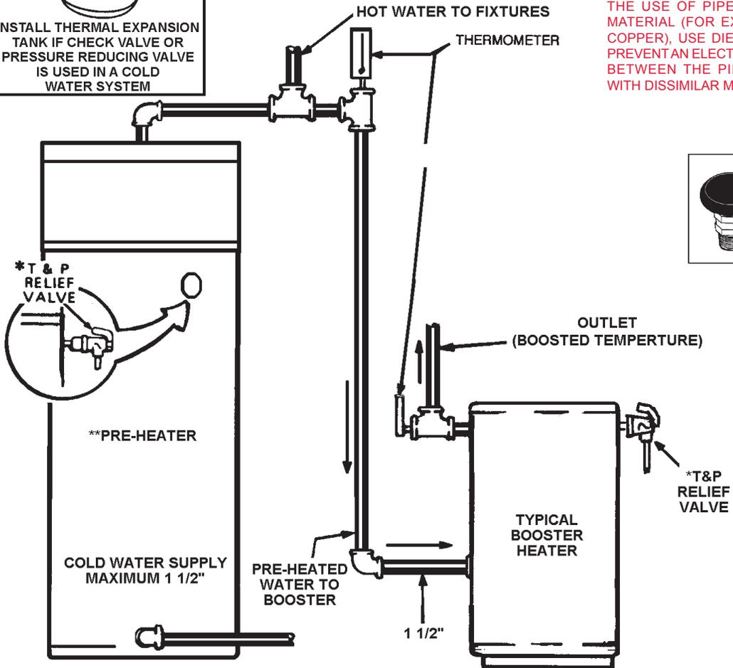
**CAUTION:** IF THE PLUMBING REQUIRES THE USE OF PIPES WITH DISSIMILAR MATERIAL (FOR EXAMPLE, STEEL AND COPPER), USE DIELECTRIC UNIONS TO PREVENT AN ELECTRO-GALVANIC ACTION BETWEEN THE PIPING COMPONENTS WITH DISSIMILAR MATERIALS.
