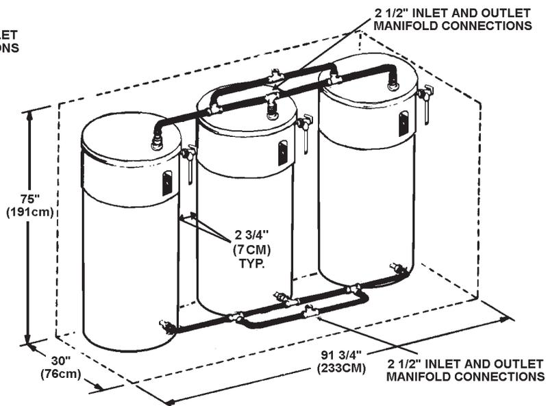
**CAUTION:** IF THE PLUMBING REQUIRES THE USE OF PIPES WITH DISSIMILAR MATERIAL (FOR EXAMPLE, STEEL AND COPPER), USE DIELECTRIC UNIONS TO PREVENT AN ELECTRO-GALVANIC ACTION BETWEEN THE PIPING COMPONENTS WITH DISSIMILAR MATERIALS.
