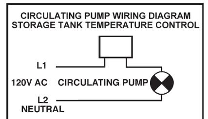
WIRING DIAGRAM FOR BOILER TO TANK LOOP AND/OR HOT WATER LOOP (IF USED).
