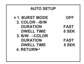
**BURST MODE** Enables (**ON**) or disables (**OFF**) the BURST (color burst) signal.
