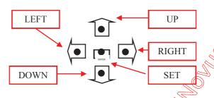
In order to enter the menu press the *SET* button. For choosing the submenus please press the *UP*, *DOWN* buttons. Enter particular sub-menus by pressing the *SET* button. To change the parameters use the *LEFT* and *RIGHT* buttons.
