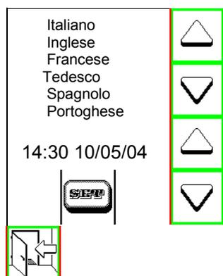
To enter the user's menu configuration, switch on the command panel by touching the display
