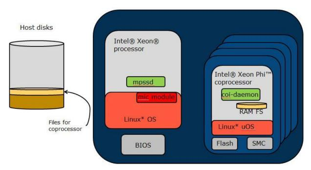
The coprocessor card contains flash and SMC (System Management and Configuration) memory which hold the BIOS, bootloader, small embedded kernel and firmware for the coprocessor. This memory does not hold the Linux microkernel. The small embedded kernel is loaded from flash when the coprocessor is initialized; the Linux microkernel is pulled over from the host when the coprocessor is booted.
