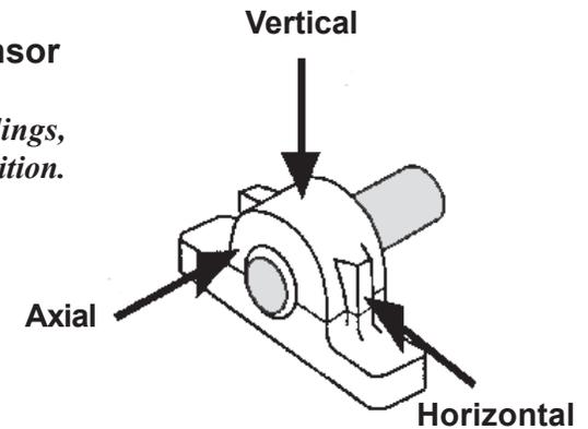
Also establish a starting point for each machine. Begin from the **OUTBOARD END** of the **DRIVE UNIT**, calling this point A. Proceed to label Points (bearings) as needed until you have reached the outboard end of the driven unit.
