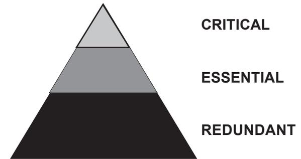
**Critical Machines** expensive premium equipment, generally >500 HP. Usually less than 5% of all plant equipment. Maintenance dollars per horsepower per year average \$11.00. This category of equipment is very well maintained and monitored. Continuous monitoring systems are better suited for this type of equipment.
