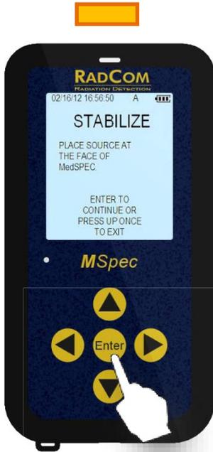
Position the Test Source on contact with the top section of the instrument during stabilization.
