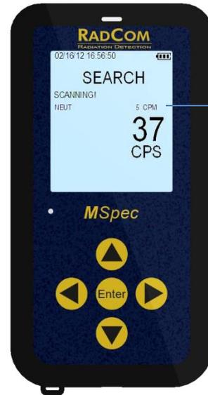
Neutron Readings Detected
