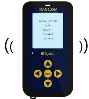
During power-up the unit vibrates, followed by the LCD displaying the welcome screen.
