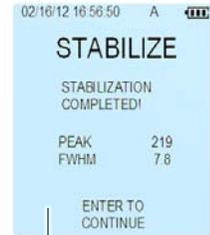
Stabilization completed. Press Enter to Finish.
