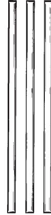
LENGTH OF HARD COPPER PIPING (SIZE OF COPPER PIPE AND SWEAT FITTINGS MUST BE THE SAME SIZE AS THE ORIGINAL PIPING.)
