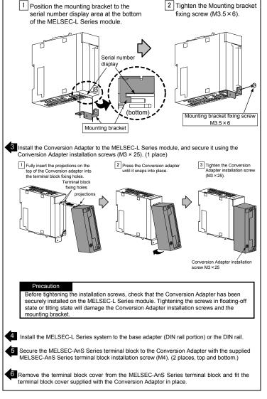
2 Secure the mounting bracket to the MELSEC-L Series module using the mounting bracket
