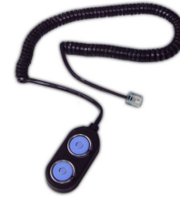
Figure 7--This DS1402D-DR8 reader, which has two receptacles for 1-Wire network testing, connects to a PC via a port adapter.
