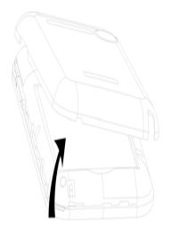
To uninstall the battery, flip the battery out from the bottom of the battery.
