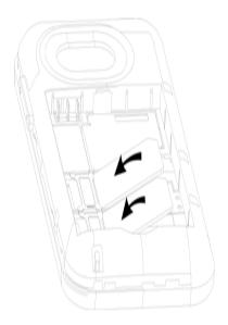
Switch off the phone, remove the back cover, battery and other external power source. Fit the SIM card into the SIM card slot. Align the angled corner of the SIM card with the slot. Slide in the SIM card, make sure it is in place, install the battery, and restore the back cover.
