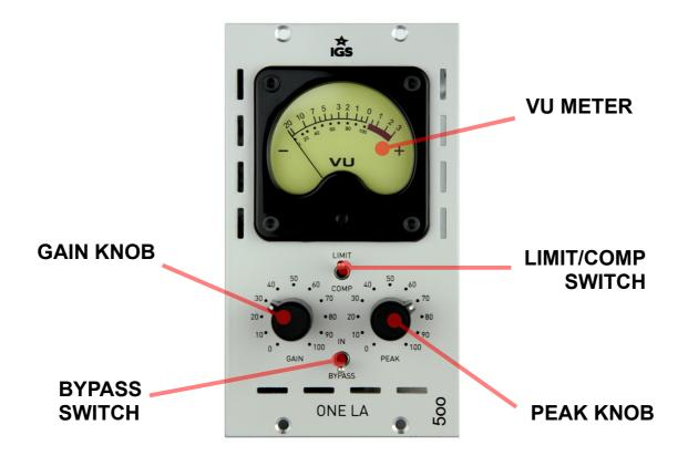
**VU METER** Clearly visible coil meter takes almost half of the space available at the front panel, to ensure that the amount of gain
