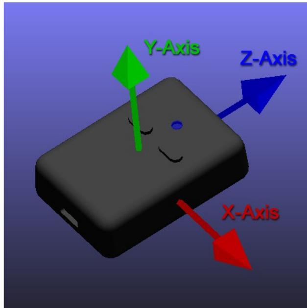
Bear in mind the difference between natural axes and the axes that are used in protocol data. While they are by default the same, they can be remapped so that, for example, data axis Y could contain data from natural axis X. This allows users to work with data in a reference frame they are familiar with.
