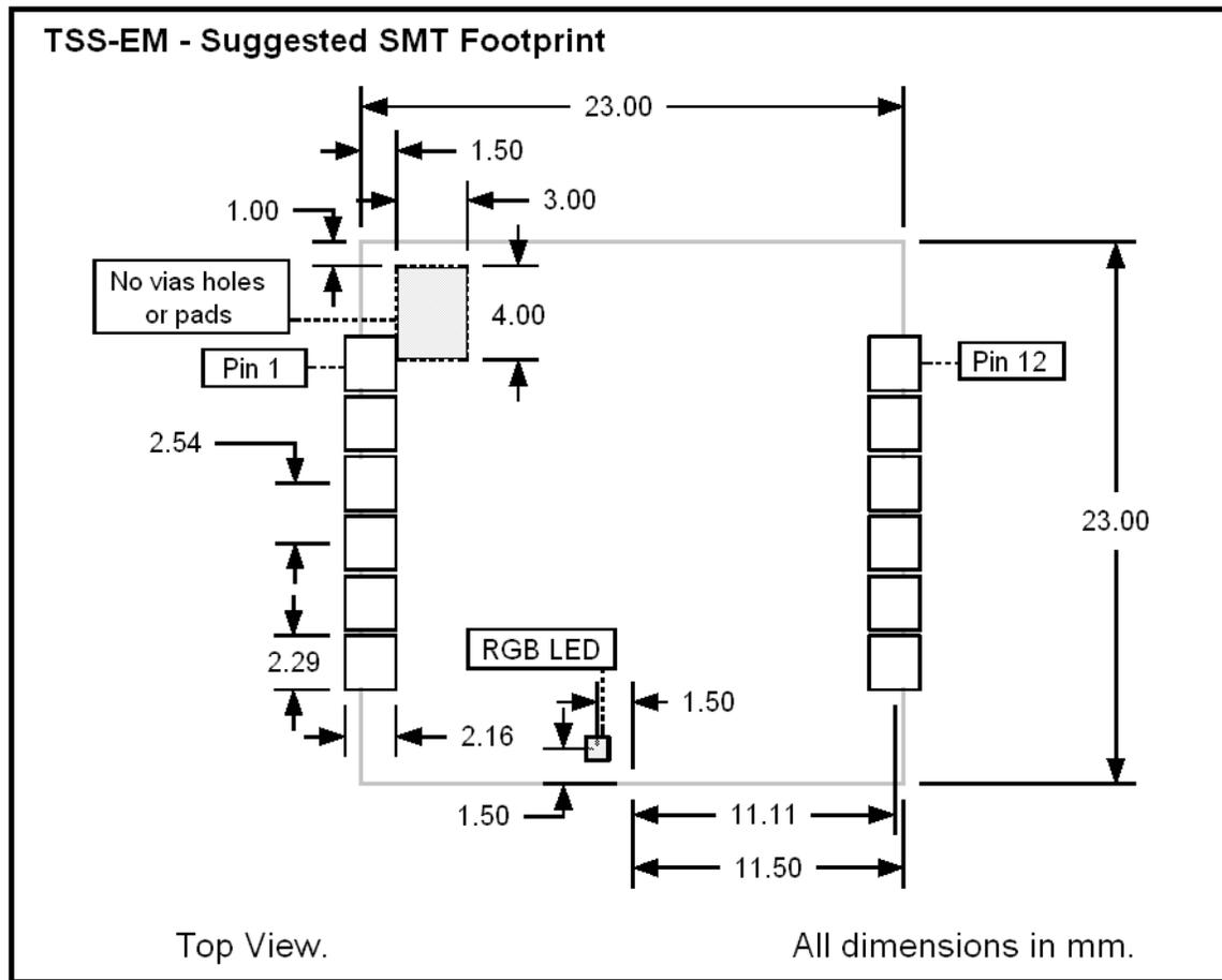
Additionally, since PCB layout can affect the performance of the 3-Space Embedded module observe the following layout guidelines:
