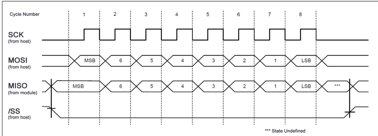
The diagram and parameter table below illustrates additional timing requirements and limits of the SPI interface:
