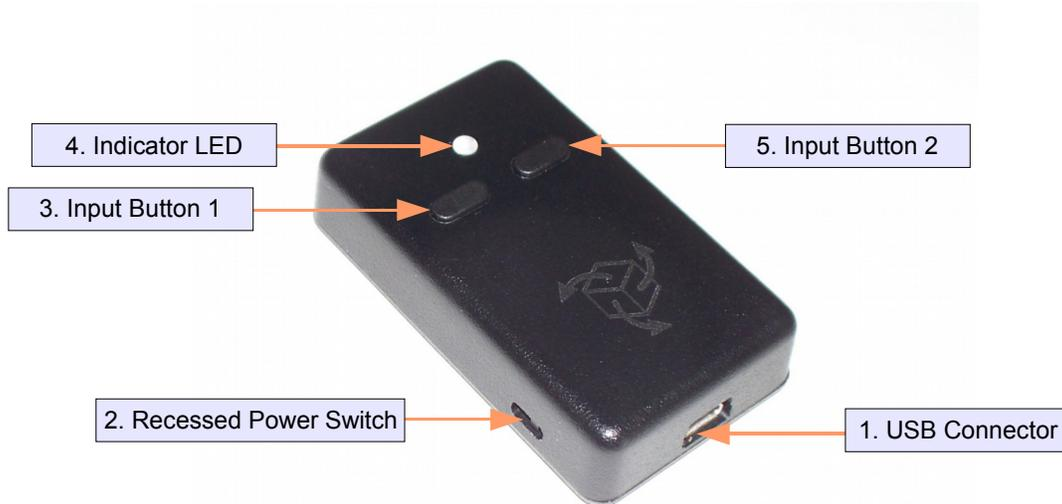
1. **USB Connector** – The 3-Space Sensor uses a 5-pin mini USB connector to connect to a computer via USB and to charge the internal battery. The USB connector provides for both power and communication signals.
