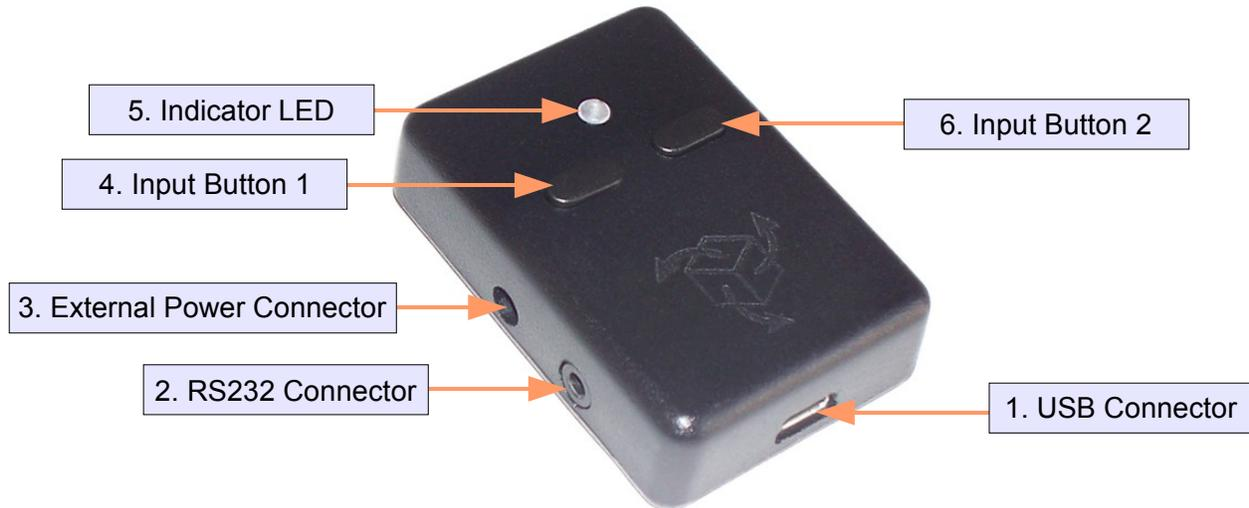
1. **USB Connector** – The 3-Space Sensor uses a 5-pin mini USB connector to connect to a computer via USB. The USB connector provides for both power and communication signals.
