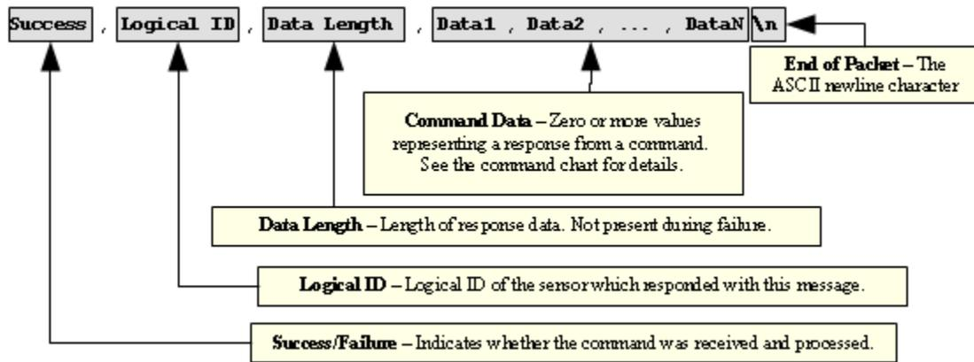
When an ASCII command is called wirelessly, before the data it would normally return in wired mode, it will return status values, each separated by a comma. First is the **success/failure value**, which is a 0 if the command was successful and 1 if it was not. Some things which can cause a failure are:
