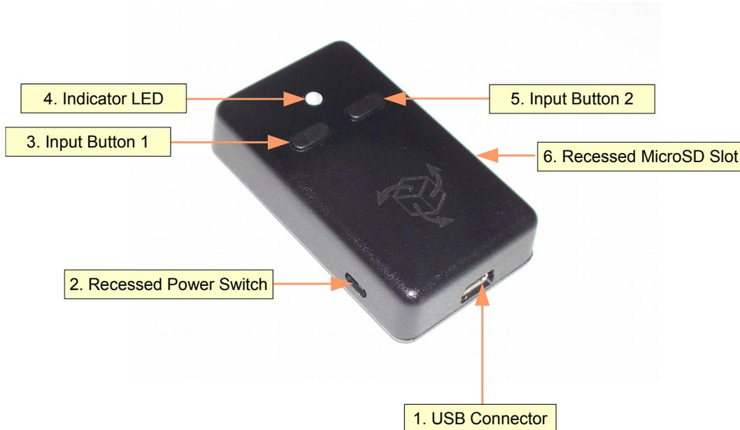
1. **USB Connector** – The 3-Space Sensor uses a 5-pin mini USB connector to connect to a computer via USB and to charge the internal battery. The USB connector provides for both power and communication signals.
