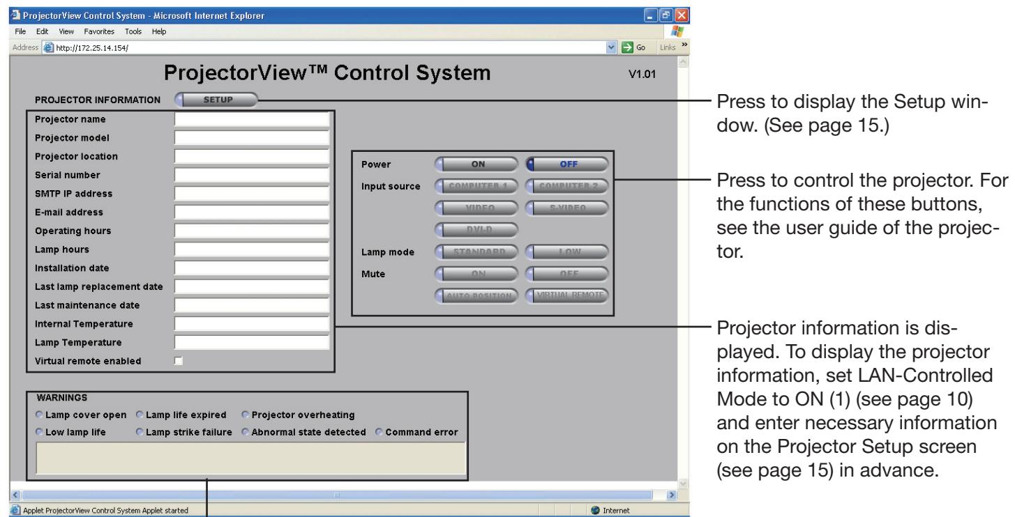
Failures in the projector are indicated with dots. When you place the mouse cursor to a dot, the indicated failure is described in the box at the bottom.
