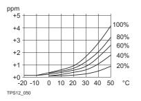
ppm % Air humidity correction [mm/km] Relative humidity [%] Air temperature [°C]
