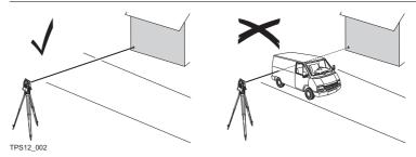
When measurements are being made using the red laser EDM, the results may be influenced by objects passing between the EDM and the intended target surface. This occurs because reflectorless measurements are made to the first surface returning sufficient energy to allow the measurement to take place. For example, if the intended target surface is the surface of a road, but a vehicle passes between the EDM and the target surface as **DIST (F2)** or **ALL (F1)** is pressed, the measurement
