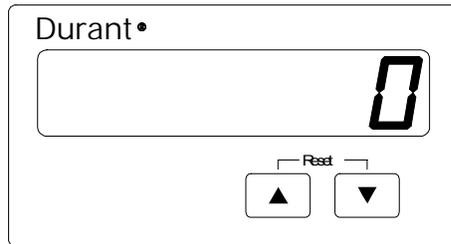
The display may or may not go to zero (or possibly the preset 2 value). That depends upon which value is being displayed, and which counter is programmed to reset via the keypad.
