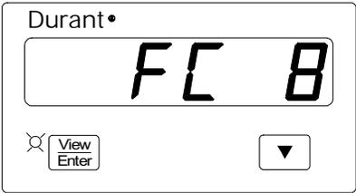
the display ascends numerically to the next FC in the list each time
