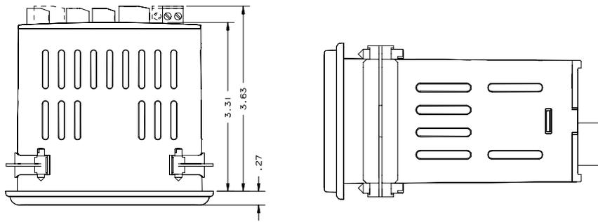
Mounting clips and screws shown in installed positions.
