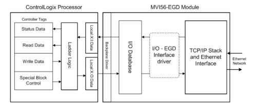
All data transferred between the module and the processor over the backplane is through the input and output images. Ladder logic must be written in the ControlLogix processor to interface the input and output image data with data defined in the Controller Tags. All data used by the module is stored in its internal database. The following illustration shows the layout of the database:
