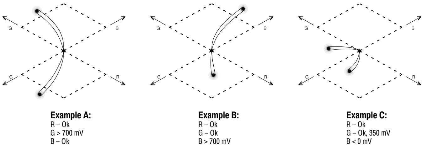
**Figure 3–23: Out-of-gamut signals on a Diamond display**
