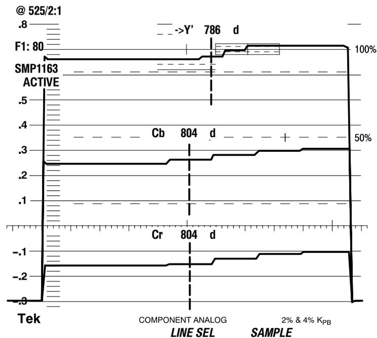
**Figure 3–15: Digital Waveform display in the VIDEO mode**
