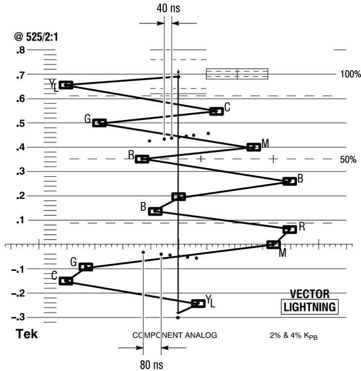
**Figure 3–39: Lightning graticule showing interchannel timing errors**
