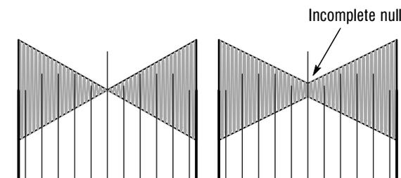
**Figure 3–10: Bowtie waveform showing gain error in CH 3**
