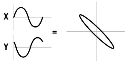
**Figure 3–5: Signals with reverse polarity and equal amplitudes**
