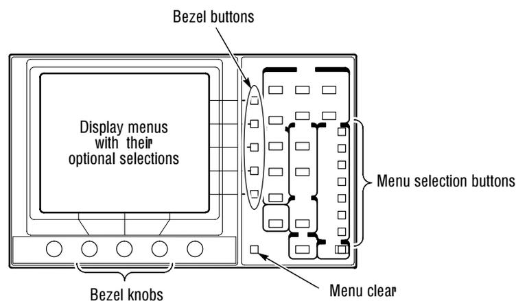
**Figure 2-3: Elements of the waveform monitor menu controls**
