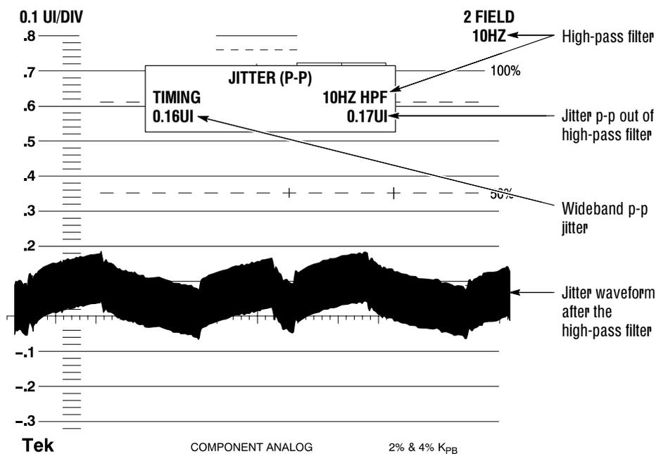
Figure 3–27: Example of the Jitter display
