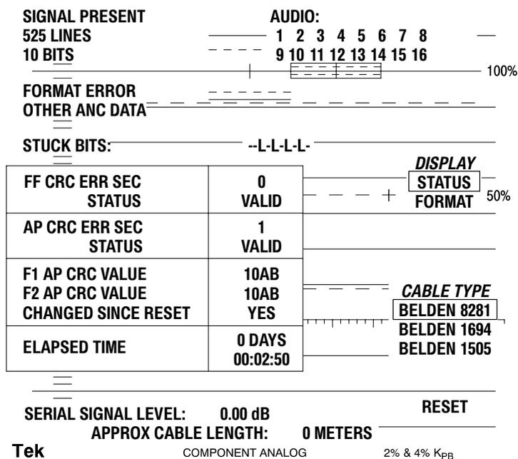
**Figure 3–32: Serial STATUS display for firmware V1.X**
