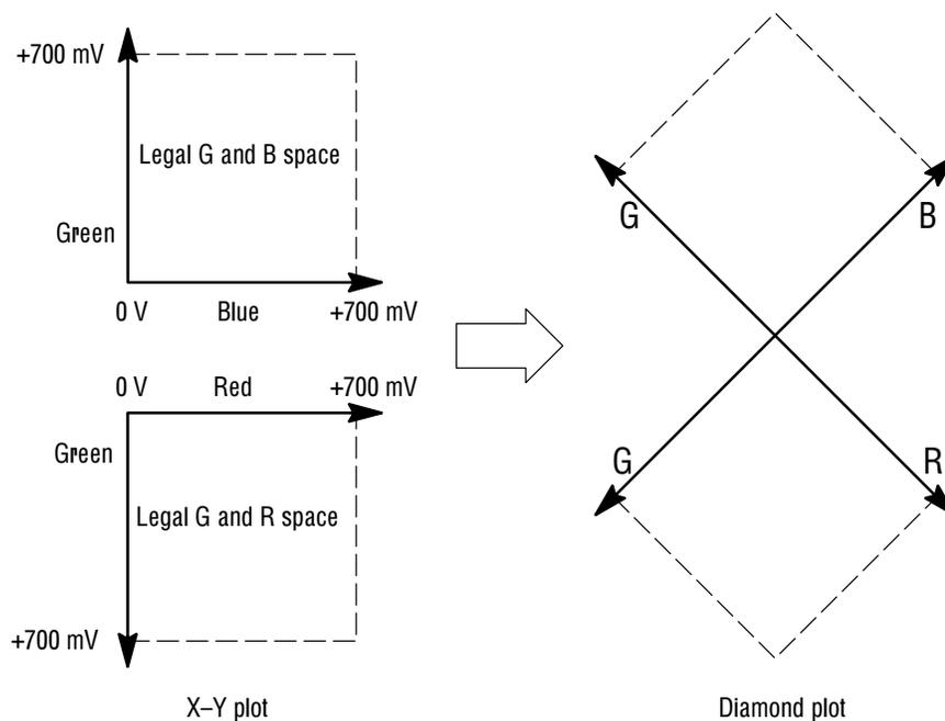
**Figure 3–22: Construction of the Diamond display**
