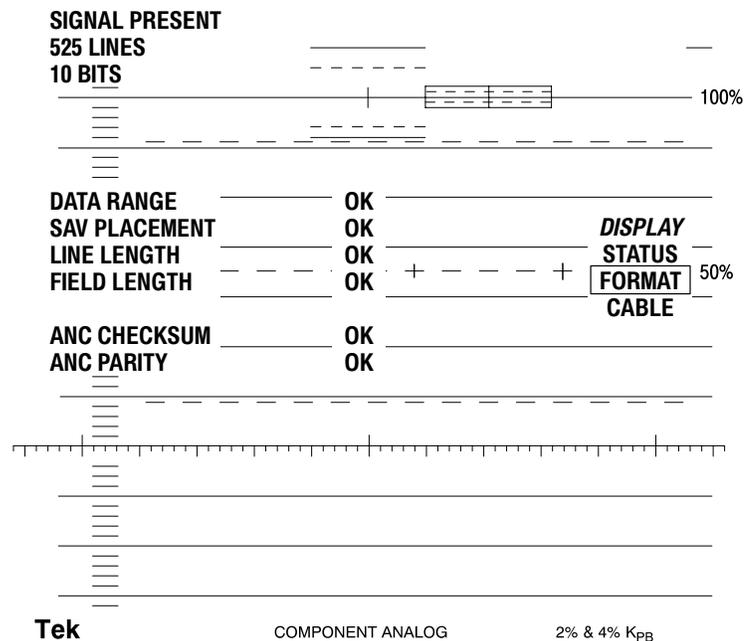
**Figure 3–33: Serial format display showing the FORMAT screen**
