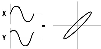
**Figure 3–3: Signals out of phase with equal amplitudes**
