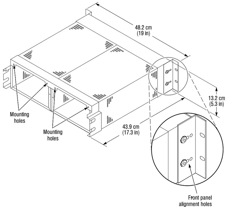
**Figure 1–4: The 1700F05 rack cabinet holds two instruments**
