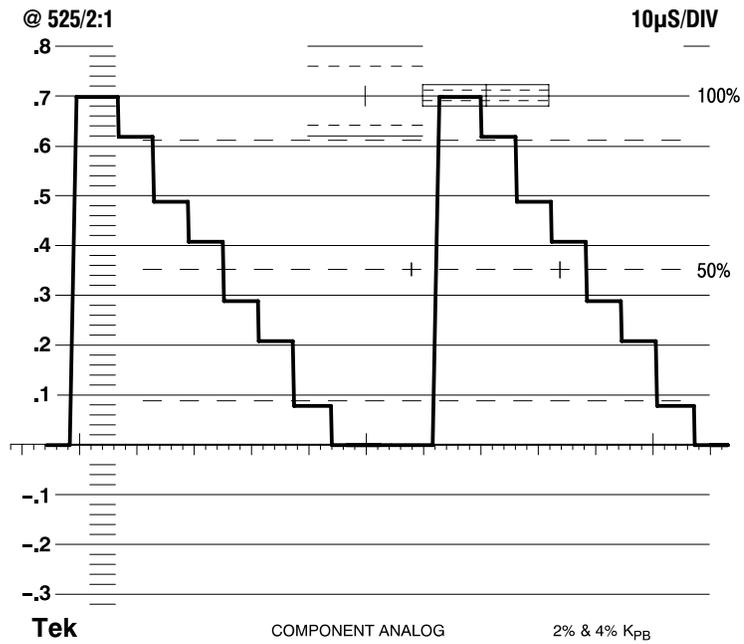
Figure 1-11: Initial display in the Waveform display mode
