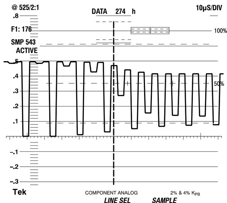
Figure 3-16: Digital Waveform display in DATA mode
