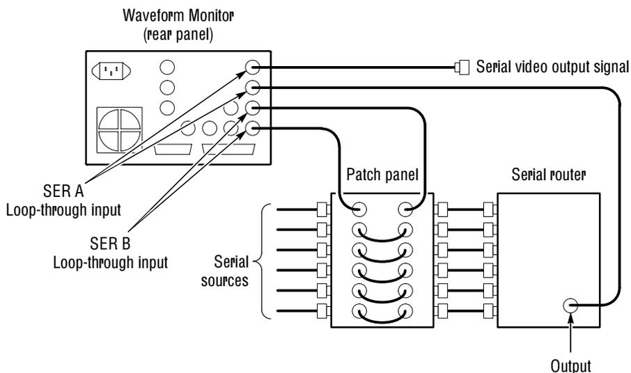
**Figure 1–7: Monitoring serial digital signals around a routing switcher**
