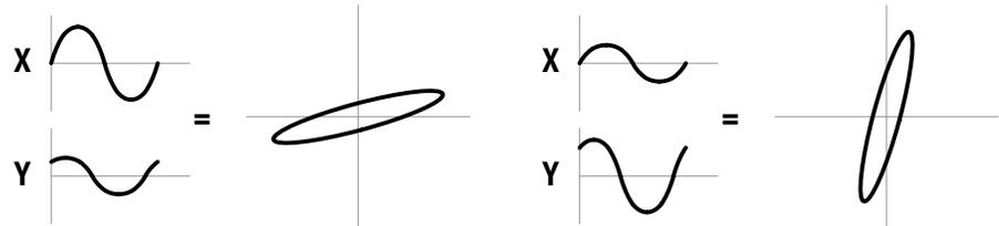
**Figure 3–4: Signals out of phase with unequal amplitudes**
