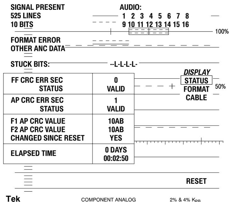
**Figure 3–31: Serial STATUS display for firmware V2.X**
