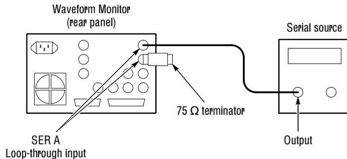
**Figure 3–20: Connections for measuring a serial source**
