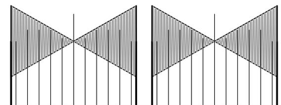
**Figure 3–8: Typical Bowtie display on the waveform monitor**
