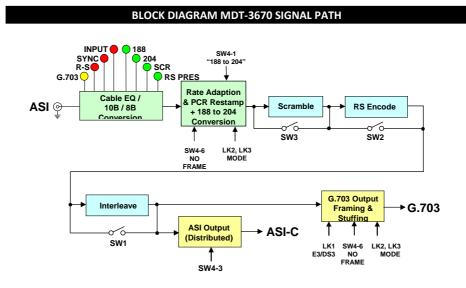
The MDT-3670 is part of a family of data transcoders for converting between the commonly used MPEG2 Transport Stream formats in the broadcast industry for video distribution.
