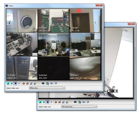
2 Select an icon (in the lower part of the window) to determine for instance the size of the views or to display the Panel window (a small window associated with the video display).
