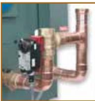
**Cold Water Start** – For applications that require reliable protection against harmful condensation caused by frequent, extended, cold water start-ups. Raypak's Cold Water Start protection system utilizes a proportional three-way valve to bypass water from the boiler outlet to the inlet during start-up, when the system return water temperature is below the minimum acceptable level. (See Cat. #1000.19)
