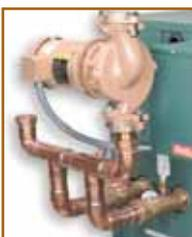
**Cold Water Run** – For applications requiring constant condensation protection. Raypak's Cold Water Run system utilizes a variable-speed pump to inject just the right amount of water from the main system loop into the boiler to maintain the optimum inlet temperature. This approach allows the full capacity of the boiler to be utilized to meet the system load, while at the same time continuously maintaining the optimum inlet water temperature to prevent condensation. (See Cat. #1000.19)
