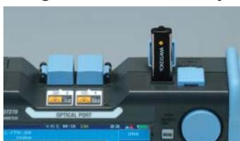
Using USB memory or a USB hard disk, you can save large amounts of data. Also, you can easily transfer saved data to a PC or other device.
