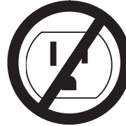
Wrong 15 Amp Outlet
