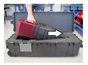
With the nose in the foam hollow, lower the back end of the EMField into the foam. Make sure the back end is flush with the foam sides.
