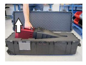
3. Continue to raise the back end of the EMField upward while moving the nose toward the back; do not lift the nose straight up.
