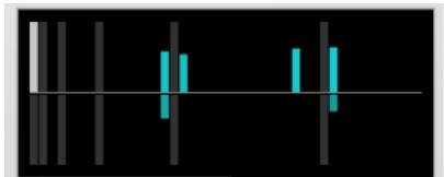
The operators have an additive synthesis engine. The operator waveform is layered at each harmonic frequency. You can edit the layering by dragging the bars in the display. The bars above the middle adjust the magnitude of the waveform at that frequency. The bars below the middle adjust the phase. For more details see the Theory section.
