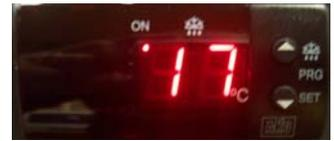
There is no need to switch the water heater off when it is not in use. The thermostat is fully automatic and only allows the gas control to open when the burner requires gas for heating. To adjust the thermostat settings refer to "[Temperature Control](#)" on page 35.
