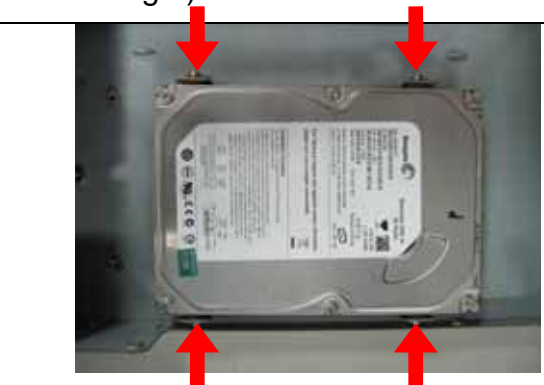
(Fig. 2-18) Fix the hard disk drive on the HDD bracket with four screws. Plug the IDE cable into hard disk drive connector
