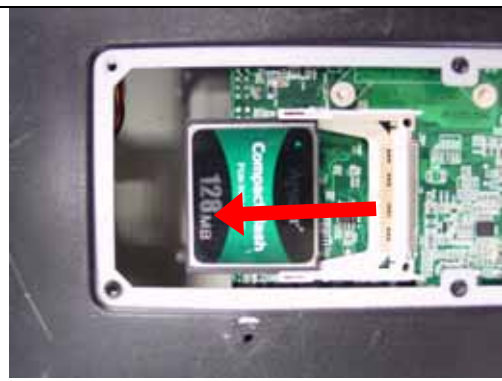
Fig. 2-14b Push CF into the bracket
