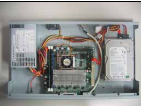
(Fig. 2-18) Fix the hard disk drive on the HDD bracket with four screws. Plug the IDE cable into hard disk drive connector
