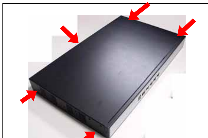
Fig. 2-3 Take off two screws
