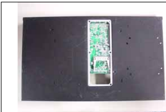
Fig. 2-14a Remove L type base under button case
