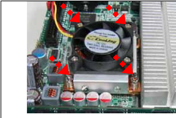
Fig. 2-7 To set up Heatsink
