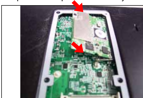
Fig. 2-16a Push Mini pci card into the bracket
