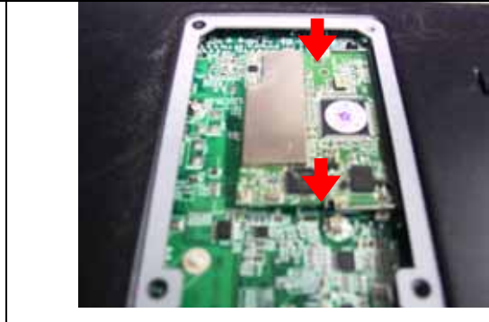
Fig. 2-16b completion Mini pci card in system
