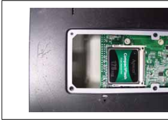
Fig. 2-15 completion CF in system
