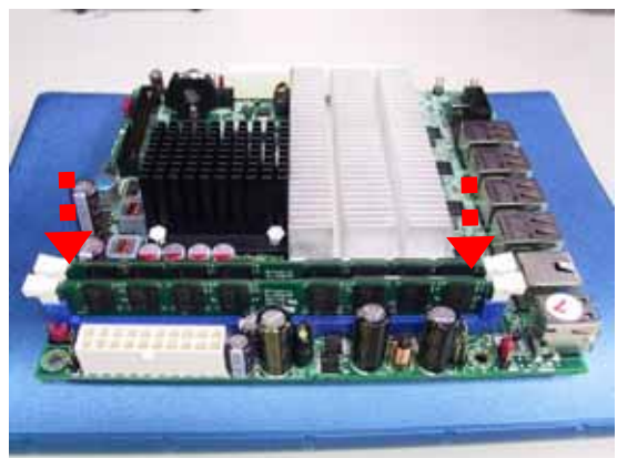
Fig. 2-10 Install Low profile DIMM
