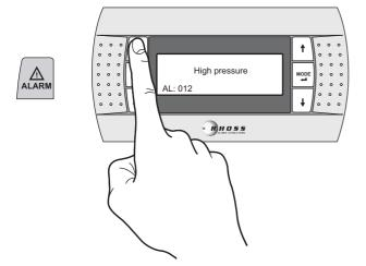
If the alarm is a type **A** alarm, it will be automatically reset. If the alarm is a type **M** alarm, you will need to press the **ALARM** key for 3 seconds to reset it. If the alarm is a type **A3M** alarm, it will be automatically reset 3 times and will then need to be manually reset.
