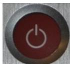
Standby. Press to switch the unit into standby mode. Press again to switch back on.
