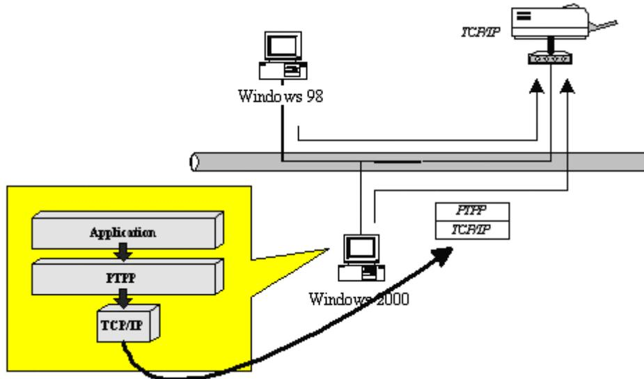
In the client installation procedure, after PTPP (Peer-to-Peer Printing Driver) is installed into Windows, the system will automatically (manual configuration is also allowed) search through all the print servers on the network, and then add their printing ports into Windows' printing port. (See below)
