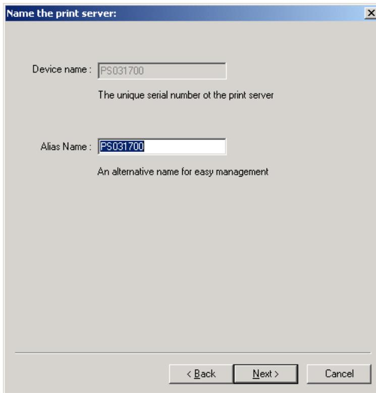
**NOTE: If this is the first time you configure the print server, the “Print Server Name” will be the same as the “Device Name” printed at the bottom of the print server.**
