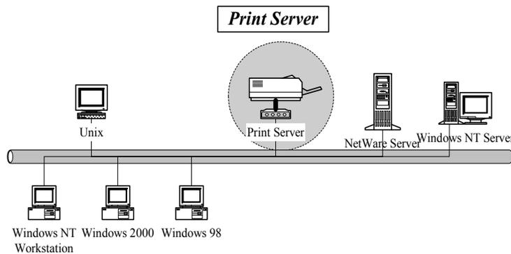
Because print server supports IPX, TCP/IP and AppleTalk network protocols, any networked computer can directly print to the print server from any of its installed protocol.
