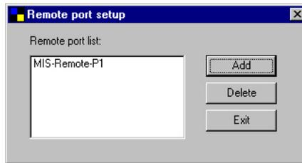
In order to use the remote printing function, you will have to proceed with normal Add Printer procedure and select your printer port as the newly added remote printer port.
