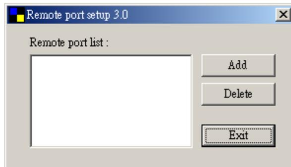
Step2. Press Add, then enter the FPS-1010's name, IP address, select used ports, and enter LPR queue name of each port.
