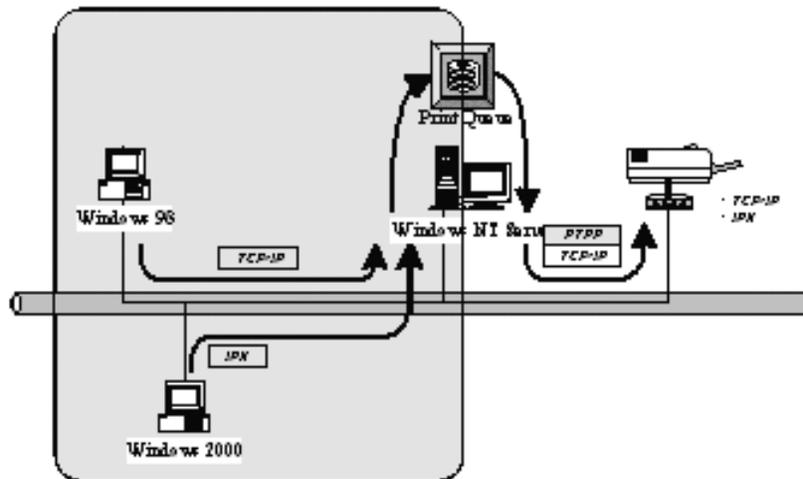
After server side's installation is completed, client side will be able to find the server's shared printer in Network Neighborhood. You only need to perform Window's standard **Add New Printer** procedure, select "**Network Printer**" shown in the screen below, and complete the configurations afterwards to access the shared printer.
