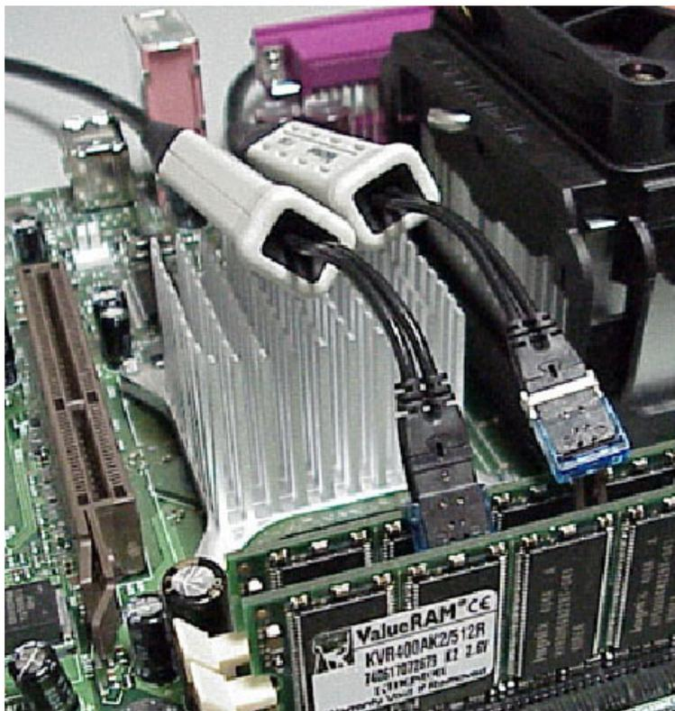
**Figure 10: Soldered Tip-Clip assemblies**
