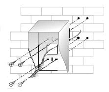
Remove the screw in the underside of the unit. Lift the aluminium cover up at the bottom and slide free. You can now access the illuminated name tag.
