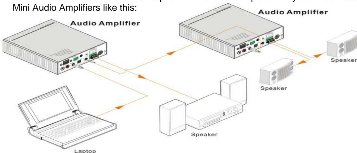
Then audio signal sent to the first Mini Audio Amplifier is cascaded to other connected Mini Audio Amplifiers, which enables multiple Mini Audio Amplifiers share the same audio source.
