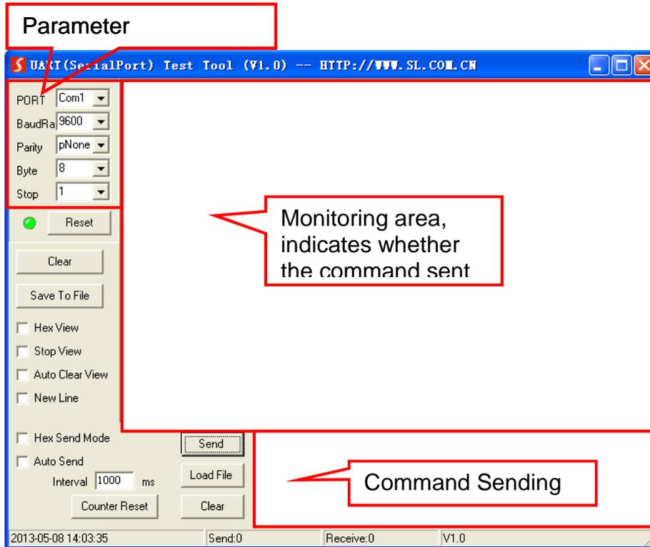
Please set the parameters of COM number, baud rate, data bit, stop bit and the parity bit correctly, only then will you be able to send commands in the Command Sending Area.
