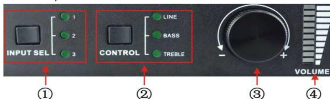
**Operation Format:** Input Sel + Control + Volume Knob (indicators and volume bar will display real-time operation)
