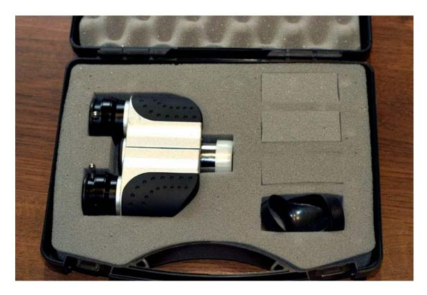
First impressions: It's a very small unit (17.5 ounces). It didn't come with any compensator lenses. It used tiny setscrews to hold the eyepieces. It had individual focusers on both sides. The casings are made of plastic.
