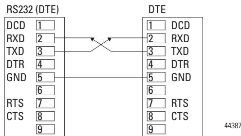
**RS232 DTE to RS232 DTE with Handshaking**
