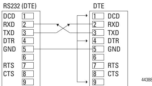
**RS232 DTE to RS232 DCE with Handshaking**
