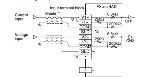
\*1 When wiring the analog output cable, use a shielded two-core twisted cable, and separate it from other power cables and cables easily affected by induction.
