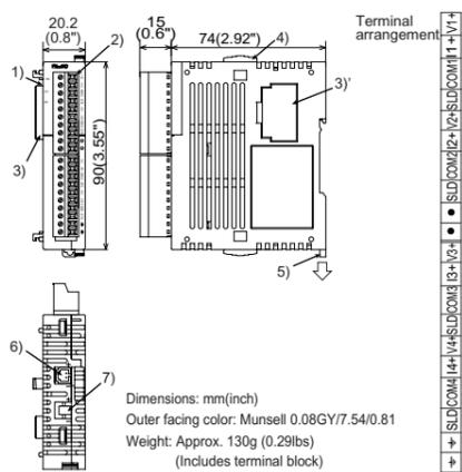
Accessory: Special function block terminal label, Power crossover cable FX2NC-10BPCB1
