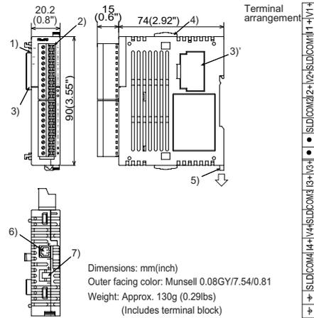
Accessory: Special function block number label, Power crossover cable FX2NC-10BPCB1
