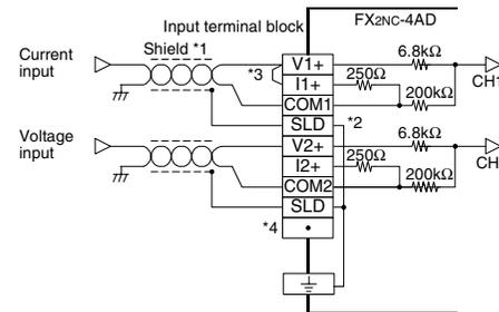
\*1 When wiring the analog output cable, use a shielded two-core twisted cable, and separate it from other power cables and cables easily affected by induction.
