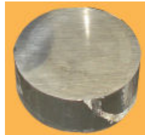
Sp10 - Cylindrical sample manufactured by a steel industry are found to have high level contamination
