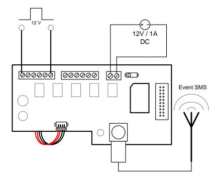
Connect one input of the configured STD35 with 12V power supply and you will get an alarm SMS to your mobile phone or an alarm e-mail to the preconfigured e-mail address (e.g. triggered by an existing alarm system, infrared sensor, temperature sensor, fluid level sensor, door contact etc.).
