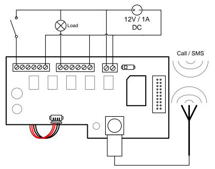
Call the configured STD35 with your mobile phone or send a SMS command and you can switch an electronic device which uses the connected power supply voltage.
