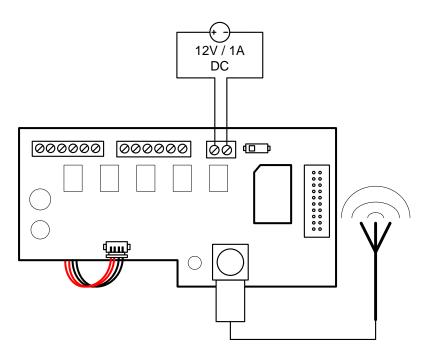
Connect the STD35 to a 12V power supply and you will receive a SMS on your mobile phone (or an e-mail to the preconfigured e-mail address) as soon as the device is booked into the GSM network. The message type is the Start-up alarm message. The power supply can be provided e.g. by a door contact or another alarm sensor.
