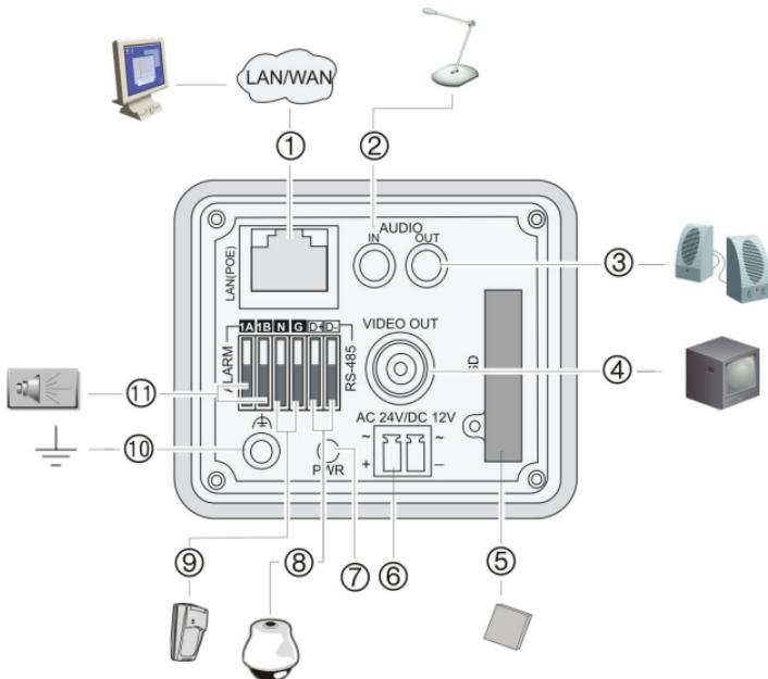
1. Ethernet RJ45 port. Connect to network devices.
