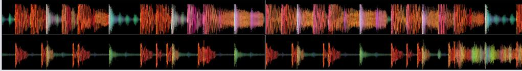
This area provides a close-up view of the track, including color-coding to show the frequency of the sound; red representing low frequency bass sounds, green representing mid frequency sounds and blue representing high frequency treble sounds. You can also switch to a three-band spectrum view by holding the control key and clicking on the waveform.
