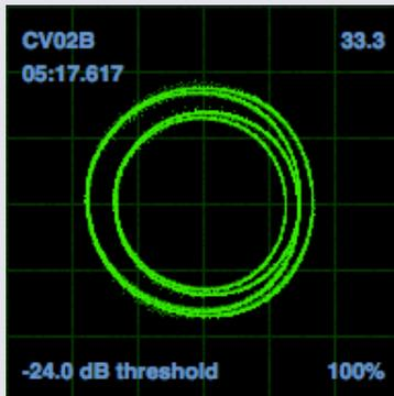
The scopes on the setup screen in Serato DJ display the input signal as a phase diagram. The key factors to look at on the scope display are crisp clean lines, round shape, and the tracking percentage in the lower right corner.
